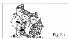
• Remove the 2 retainer from the spool valve case, and remove the spool valve case. [Fig.7.1]
