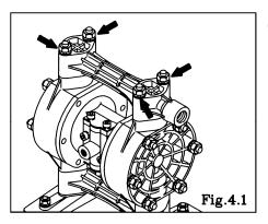
• Remove the 4 retainer nuts from the out manifold, and remove the out manifold. [Fig.4.1]
