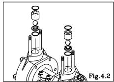
• Remove the O ring, valve stopper, ball (flat valve) and valve seat. [Fig.4.2]
