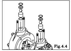
• Remove the O ring, valve seat, ball (flat valve) and valve stopper. [Fig.4.4]
