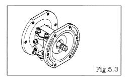
Remove the center disk and diaphragm from the opposite side using the double nut. [Fig. 5.3]
